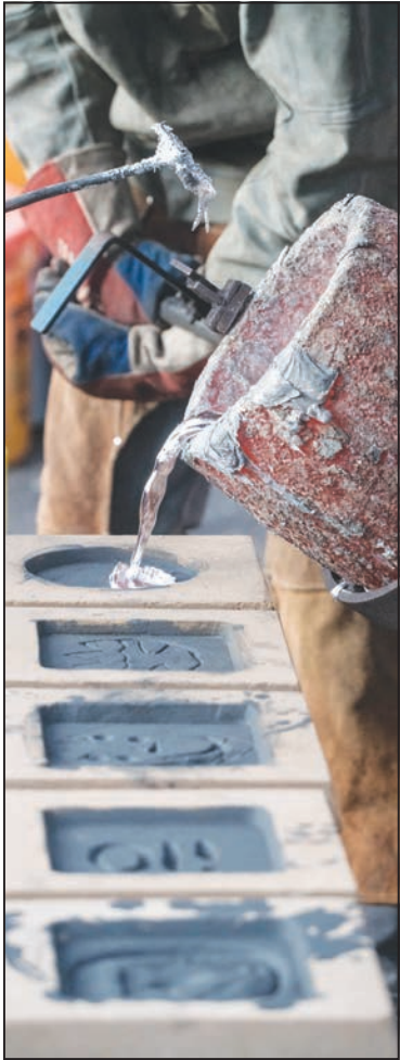
Molten aluminum is poured into molds.
